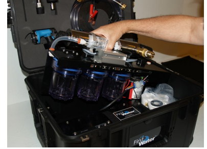
Replace filter housing
